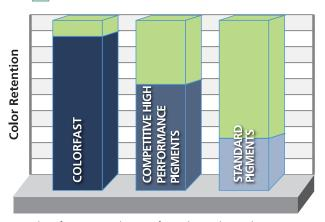
Results after 10,000 hours of Accelerated Weathering and Light Fastness (ASTM G153)
