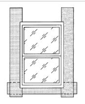
8. Installing the Window: After the strips of Water-Resistive Barrier have been installed at the sill and jambs as shown, the window can be installed (Fig 22.9).
