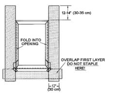
7. Installing Water-Resistive Barrier at Jambs: Fold Water-Resistive Barrier into rough opening. Bottom leg must overlap first layer. Do not staple immediately below the sill/jamb corners (Fig 22.8).
