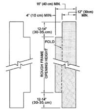
**6. Cutting Water-Resistive Barrier for Jambs:** Cut Water-Resistive Barrier to fit rough opening jamb (Fig 22.7).
