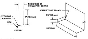
9. Metal Flashing Profile: The flashing above the window should be fabricated in the profile shown. Flashing material should be corrosion resistant and compatible with other construction materials (Fig 22.10). The length of the cap flashing must be at least as long as the top of the window and may be up to 1/2 in. (13mm) longer at each end when installed (not mandatory).
