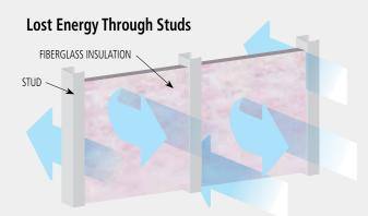
opportunity for energy to flow in and out of the building. Climate controlled air escapes and uncontrolled air invades the building, requiring the building's HVAC system to use more energy to maintain the desired temperature.
