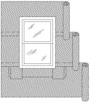
STEP 12: INSTALLING ROLLS OF WATER-RESISTIVE BARRIER CONT.
