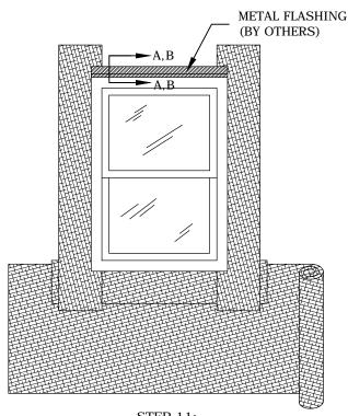
STEP 11: INSTALLING ROLLS OF WATER-RESISTIVE BARRIER
