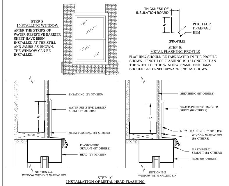
LENGTH OF THE FLASHING IS DEPENDENT ON THE TYPE OF WINDOW USED. SECTION A-A & B-B ILLUSTRATE TWO TYPES OF WINDOWS. FLASHING SHOULD BE INSTALLED AS ILLUSTRATED. FOR ANY UNUSUAL CONSTRUCTION PLEASE CONTACT PAREX USA TECHNICAL SERVICES.
