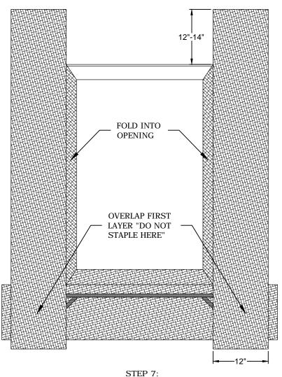
INSTALLING WATER-RESISTIVE BARRIER SHEET AT JAMBS FOLD WATER-RESISTIVE BARRIER SHEET INTO ROUGH OPENING. BOTTOM LEG MUST OVERLAP FIRST LAYER AS SHOWN. DO NOT STAPLE IMMEDIATELY BELOW THE SILL JAMB CORNERS.
