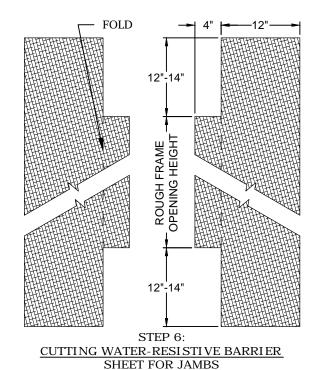
CUT WATER-RESISTIVE BARRIER SHEET TO FIT ROUGH OPENING JAMB.
